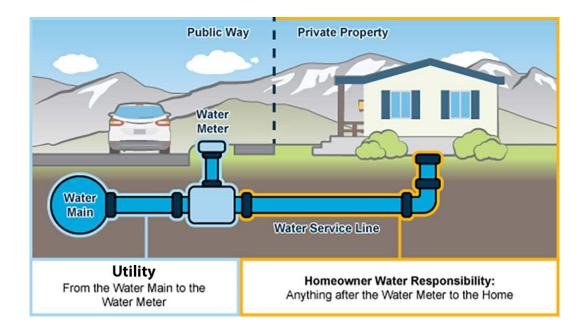
If determined that you have a Galvanized Service Line, please consider replacing it in its entirety. This is the best way to reduce lead in your water. Homeowners must contract individually with a licensed plumber to have the service line replaced from the meter to the house. Coordinate with the Water District for replacement of the District owned portion of the service line at the same time.
